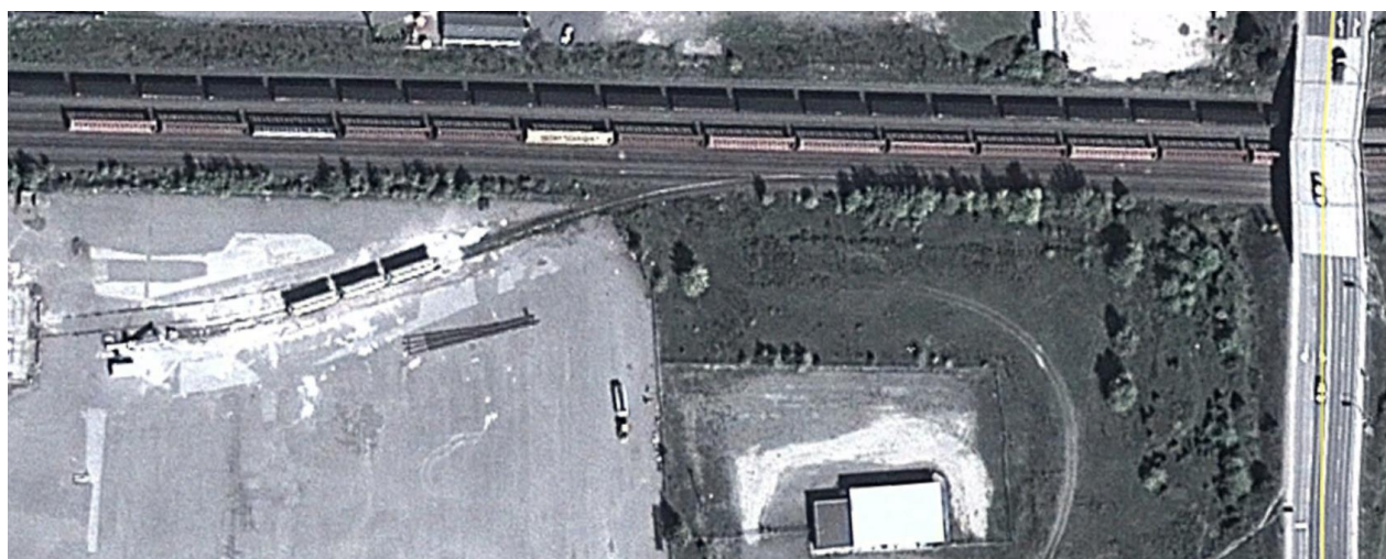
Figure 4-7: Existing Rail Spur Used for Cement Transloading in Terrace
