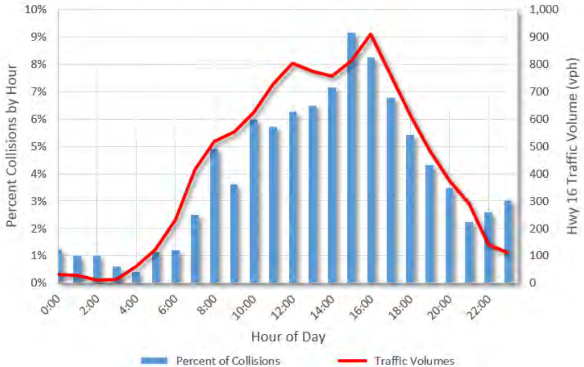
Figure 48: Percent of Collisions and Traffic Volume by Hour of the Day (Source: MoTI Count Station 48-923EW on Highway 16 at Kenney Street, July 2014)
